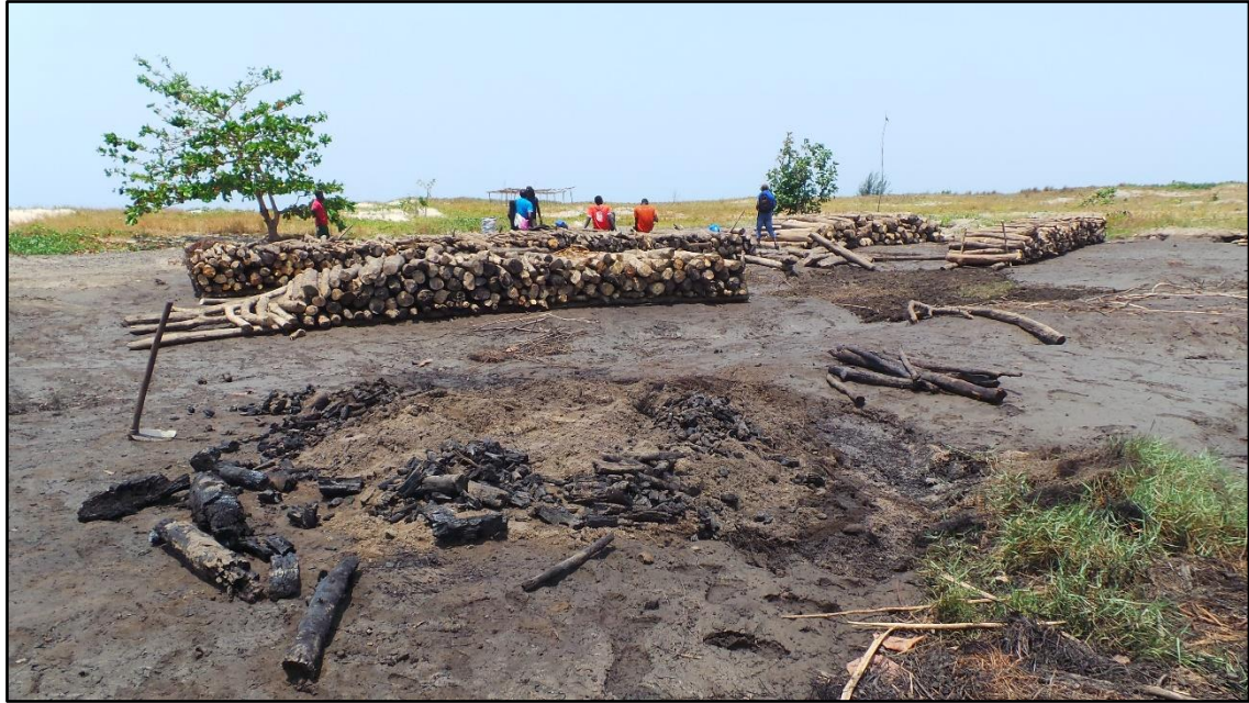
Figure 35: Field of ovens for production of charcoal (Ponta Liberal, coastal bar of Chinde river mouth) [Díaz P., I.; Oct. 2017].
