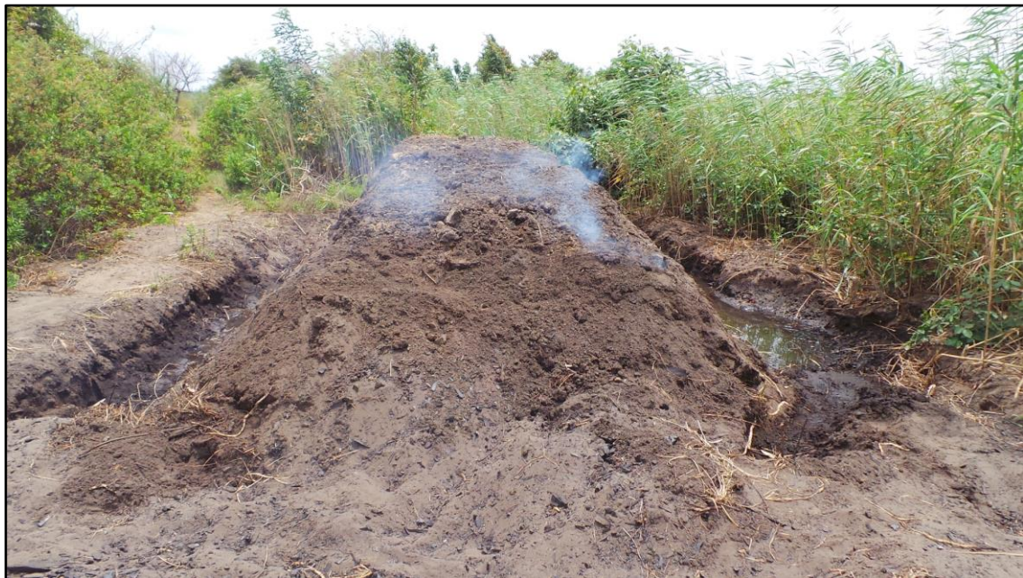
Figure 37: Usually, charcoal producers dig channels around the oven connected to a local stream. Once the charcoal material has been removed, they use the water from the peripheral channel to extinguish the oven [Díaz P., I.; Oct. 2017].
