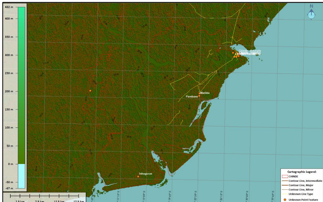
Figure 5: Digital Elevation Model (DEM) and hypsometry of Administrative Post of Chinde. Cartographic Source: Global Mapper, ASTER GDEM v2 Worldwide Elevation Data (1 arc-second resolution).
