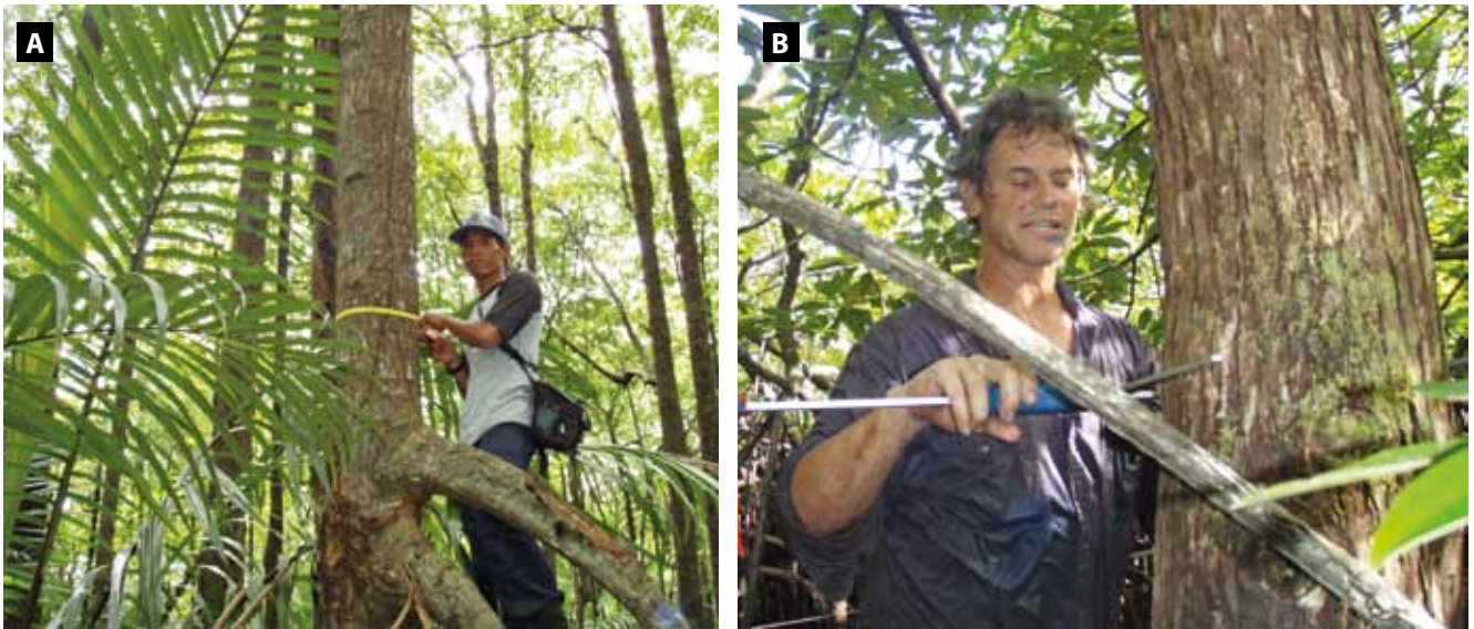
Figure 12. Measuring tree diameter at breast height (Left photo by Dan Donato/University of Wisconsin; right photo by Chris Heider/Watersheds Professional Network)
